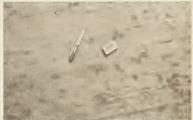
FIGURE 15.—ILLUSTRATION OF THE CLOSED TEXTURE CHARACTERISTIC OF MOST OF EXPERIMENT 3. ANALYSES OF MAT AND OF UNDERLYING SUBGRADE AT STATION 353 ARE GIVEN IN TABLE 7.
